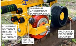
Positioning of each wheel scanner is accomplished by mechanical adjustments.
