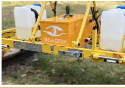
The design includes the system of constant dynamic track gauge repetition whereby the measuring wheel (RSUI) is always in the optimal position relative to the rail head during the inspection.
